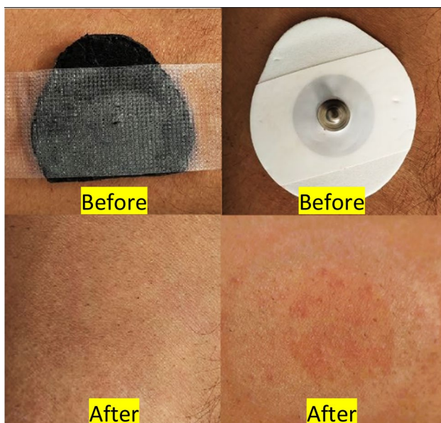
Fig. 12 Skin reaction comparison of (a) CNT/PDMS sheet and (b) Ag/AgCl electrode (Color figure online).
